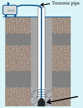
Grout filling well from the bottom to top.
