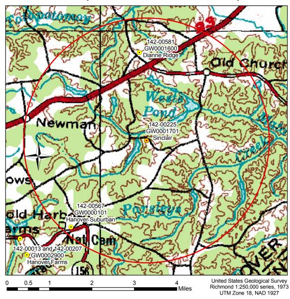
Area of Impact based on 2-d analytical simulation of a single confined aquifer. Pumping was simulated at 5,310,000 gallons per year for 10 years. Transmissivity of 610 ft sq/day was estimated from an on-site step test. Storage coefficient was estimated from a nearby aquifer test. The one-foot drawdown contour (area of impact) occurs at 15,260 ft from the pumping well.
